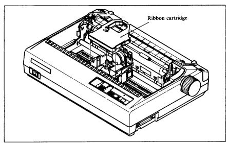
Figure 5-1. Replacing the ribbon cartridge
