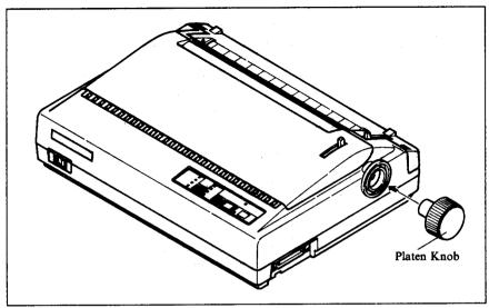
Figure 1-3. Mounting the platen knob
