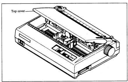
Figure 1-4. Removing the top cover
