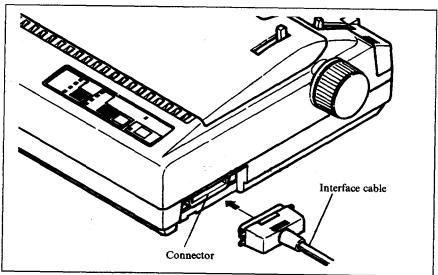
Figure 1-6. Connecting the interface cable
