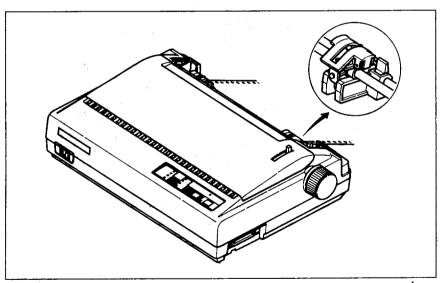
Figure 1-11. Closing the sprocket covers
