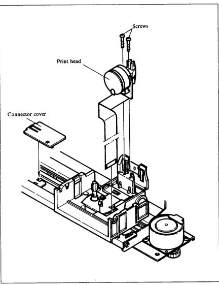
Figure 5-2. Replacing the print head
