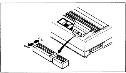
Figure 1-15. DIP switches
