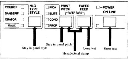
Figure 2-4. Power-up functions of control panel
