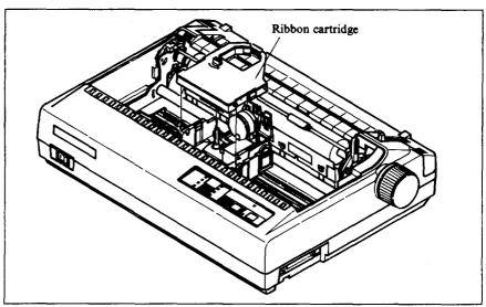
Figure 1-5. Installing the ribbon cartridge
