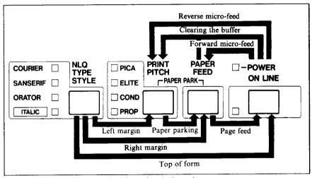
Figure 2-7. Switch combination functions of control panel
